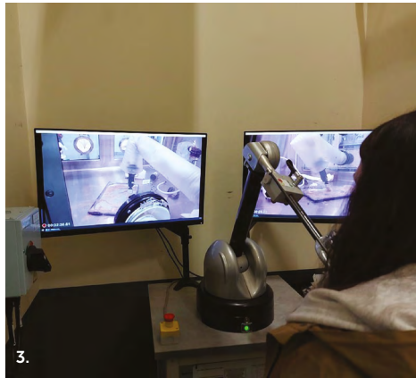
1. Demonstration of the Kinova robotic arm in a nuclear glovebox
