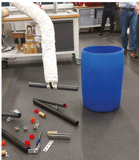
1-3. Proof-of-concept demonstration of the inflatable robotic arm in the Engineering Centre of Excellence at Cleator Moor on 21st February 2024
