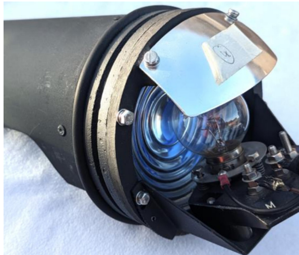
Figure 24: Bulb and lens module used in filament JIs.
