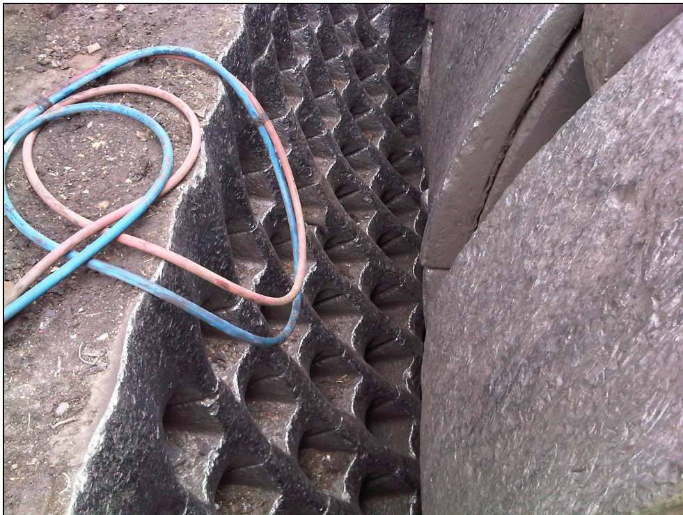
Picture 3 - Example of bottom grids through which fragmentised scrap is forced. The uneven surface of the grid is due to material wear abrasion.
