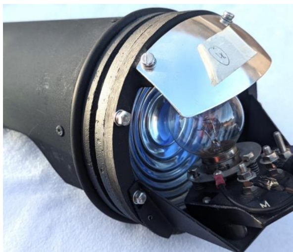
Figure E2: Bulb and lens module used in filament junction indicators.
