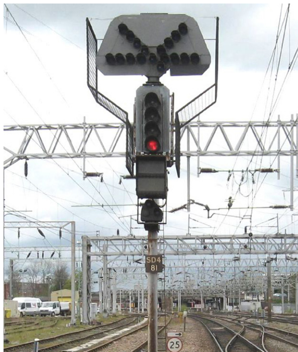
Figure E1: Example of a junction indicator
