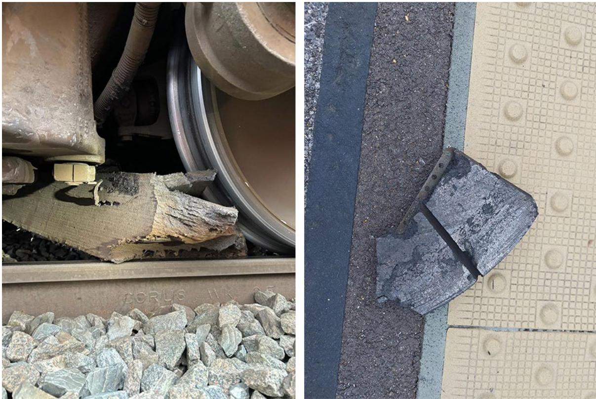
Remains of the temporary RRAP found under train 1R00 (left) and the brake pad found on Kings Langley station platform (right) (courtesy of Network Rail).
