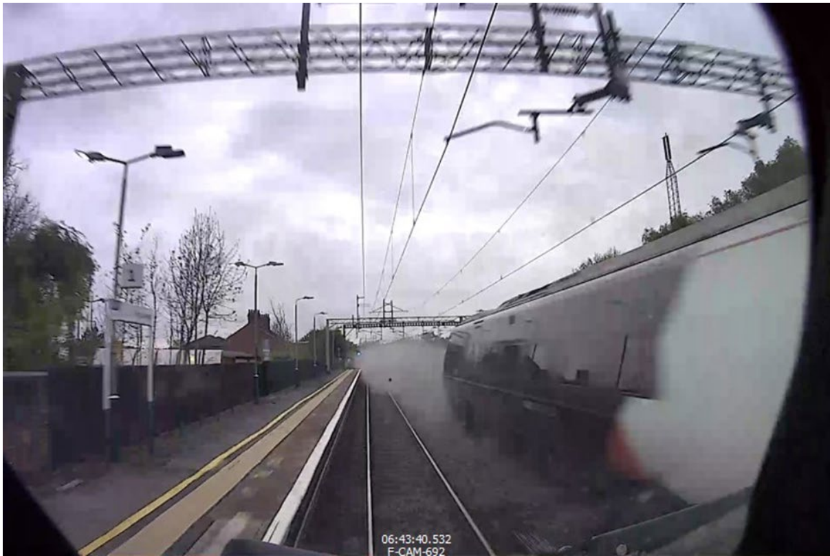
Forward-facing CCTV from 9S44 as it passes 1R00 through Kings Langley station. A dust cloud and debris is evident from the rear of 1R00 (courtesy of Avanti West Coast).
