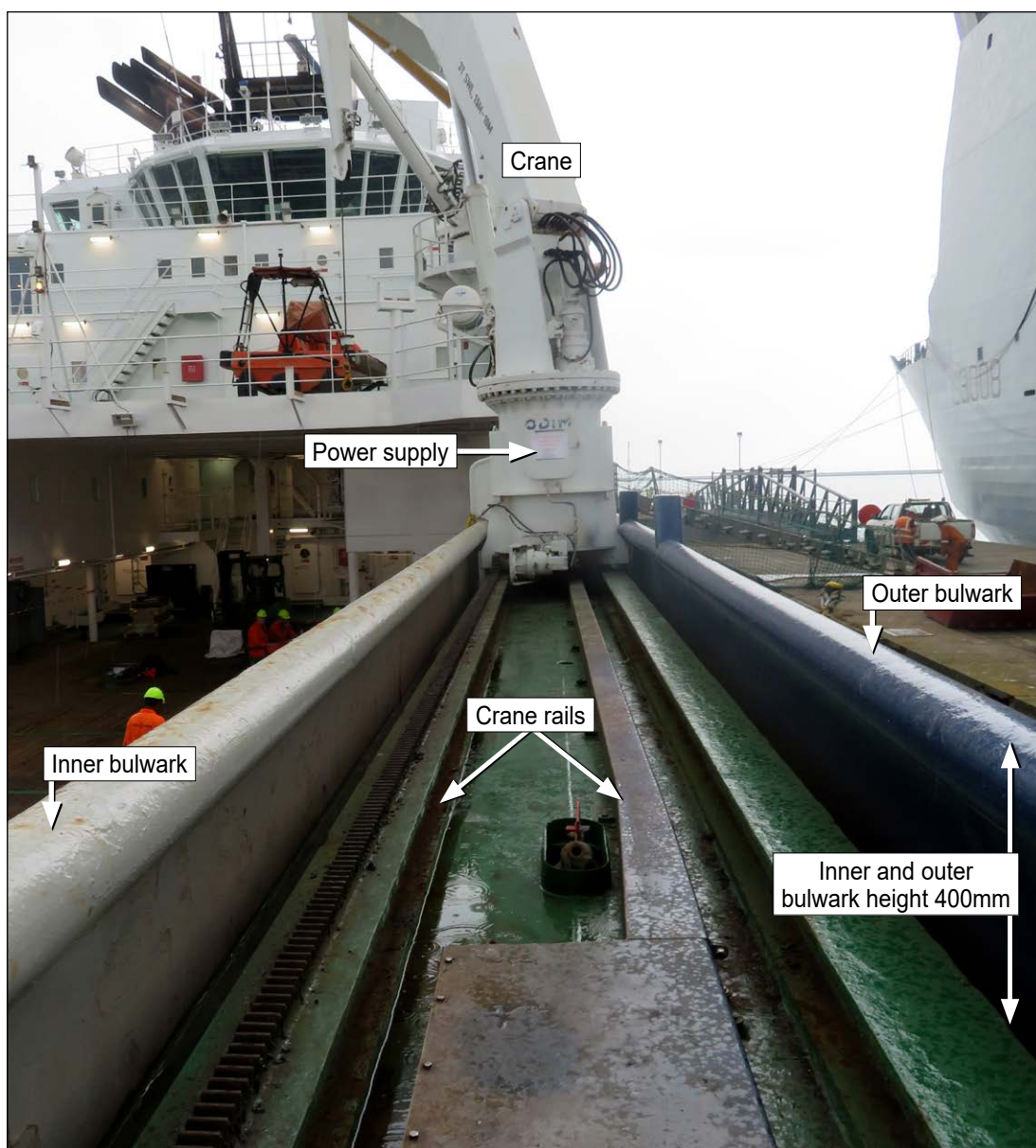
Figure 2: Starboard rail-mounted crane
