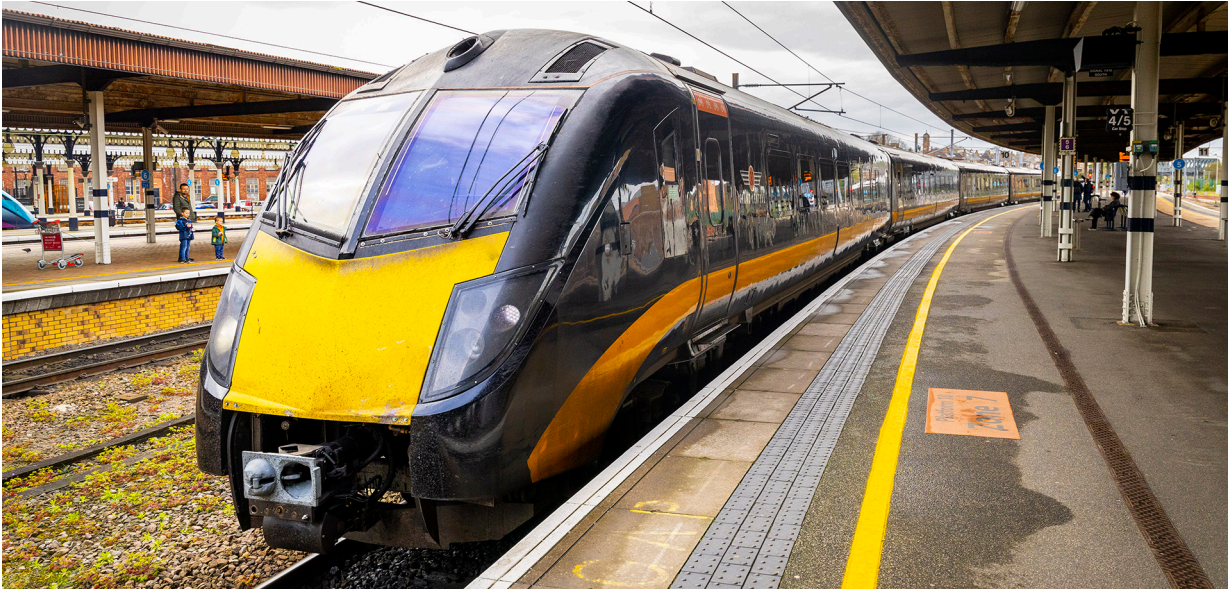
Figure 3: Grand Central class 180 diesel-hydraulic multiple unit (courtesy of Grand Central).
