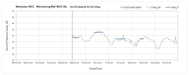
Note: Missing data between the start of the month and 10:00 on Wednesday 03<sup>rd</sup> of July was due to a communication error between the monitoring station and the server.
