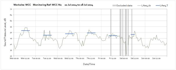
Note: Missing data between 03:00 and 05:00 on Saturday 27<sup>th</sup> July was due to a communication error between the monitoring station and the server.
