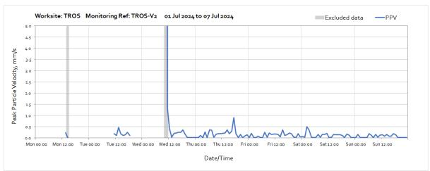
Note: Missing data throughout the week was due to a loss of power to the monitoring station caused by vegetation preventing sufficient light reach the solar panel.
