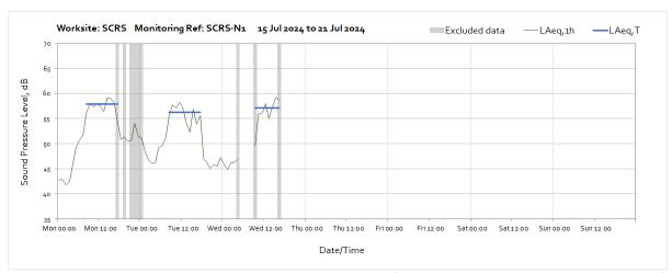
Note: Missing data between 05:00 and 08:00 on Wednesday 17<sup>th</sup> July and between 17:00 on Wednesday 17<sup>th</sup> July and the end of the month was due to a loss of power to the monitoring station caused by poor weather conditions preventing sufficient light reach the solar panel.
