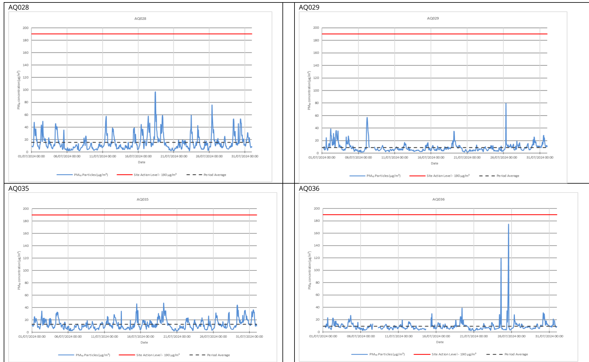
Figure 3: Construction dust 1-hour mean indicative PM 10 concentration for all dust monitors
