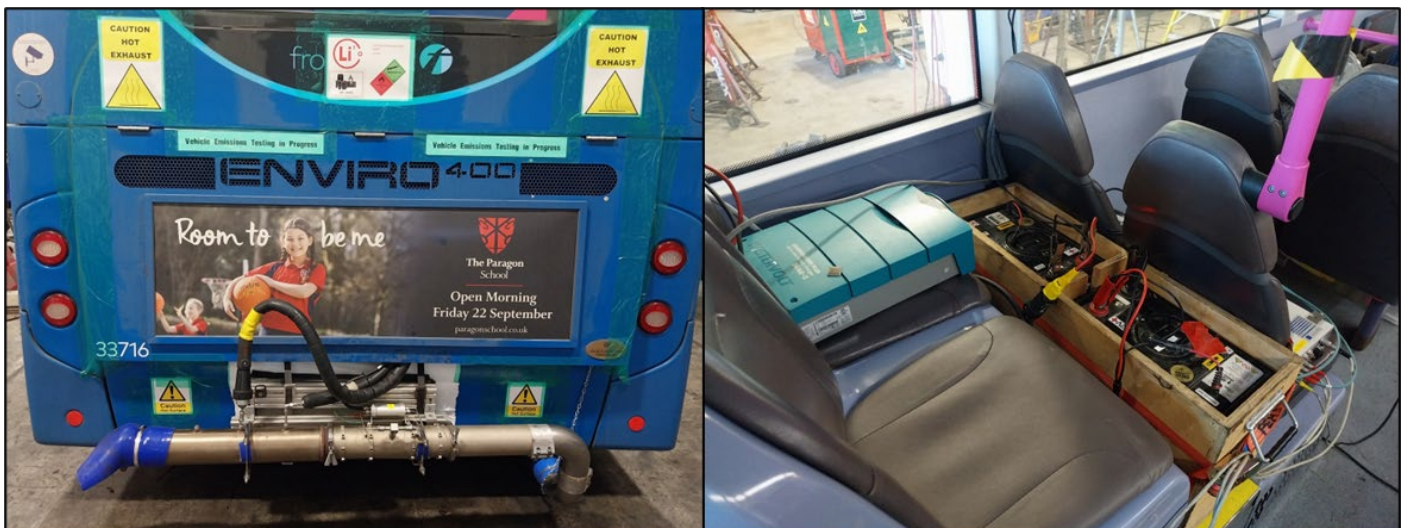
Figure 4 PEMS equipment in use (taken on a bus in Bath, September 2023).
