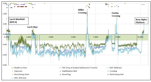
Figure 3-6: PL1531 4" GL Pipeline Burial Profile (2014 & 2018)
