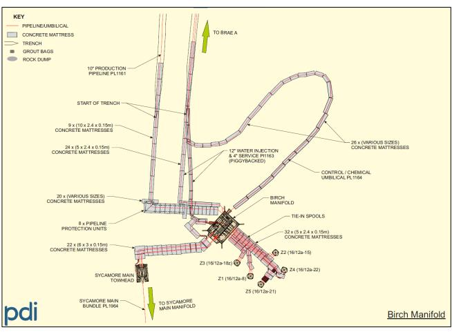
Figure A-5: Birch Manifold and Wells
