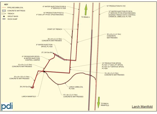
Figure A-4: Larch Gas Lift (& Production) Manifold & Wells
