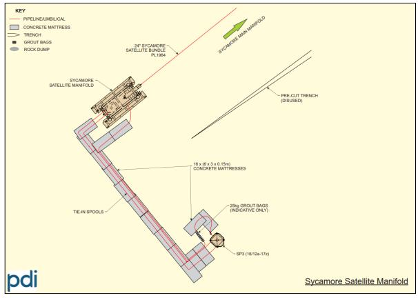
Figure 1.8.7: Sycamore Satellite Manifold & Wells
