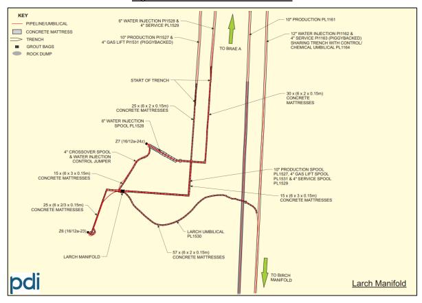
Figure 1.8.5: Larch Gas Lift (& Production) Manifold & Wells
