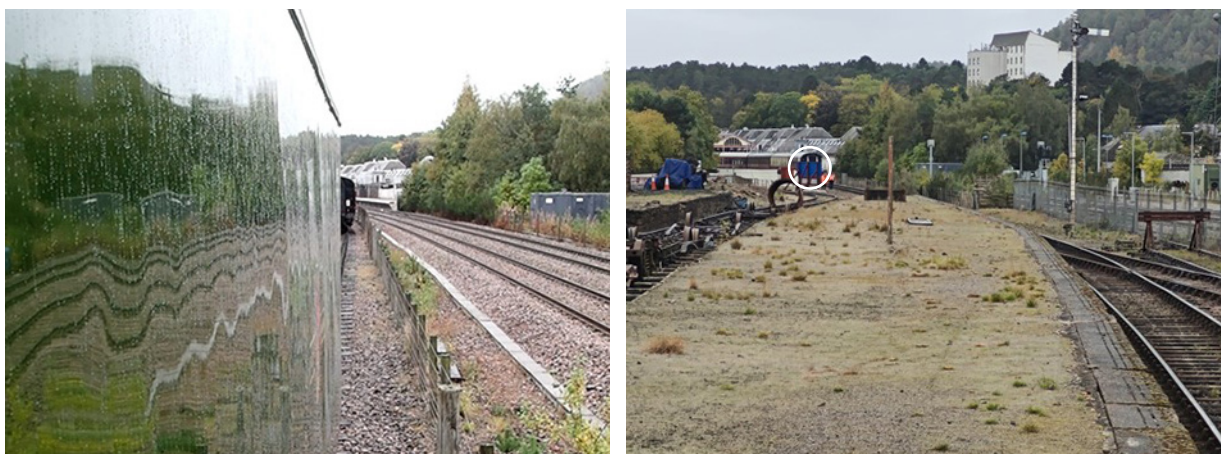
Figure 8: The view along the driver's side of the tender when the locomotive is 62 metres from the coaches (left) contrasting with the view along the fireman's side at Speyside (right) with the position of coach end (circled).
