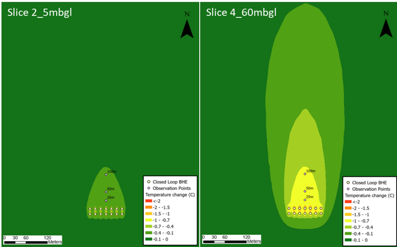
Figure 4-1: Extent and temperature change of the simulated thermal plume after 50 years for a heat extraction scenario at 5m and 60m bgl.
