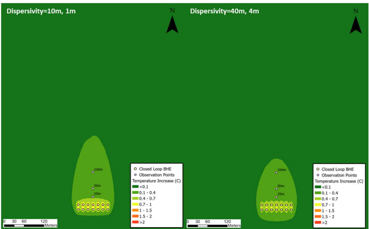
Figure 3-20: Extent and temperature change of the simulated thermal plume after 50 years for different dispersivities, at 5m bgl (slice 2)
