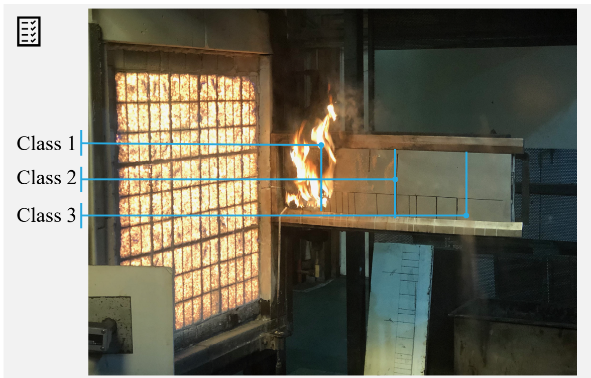
Figure 5.2: Image of BS 476-7 test in operation
