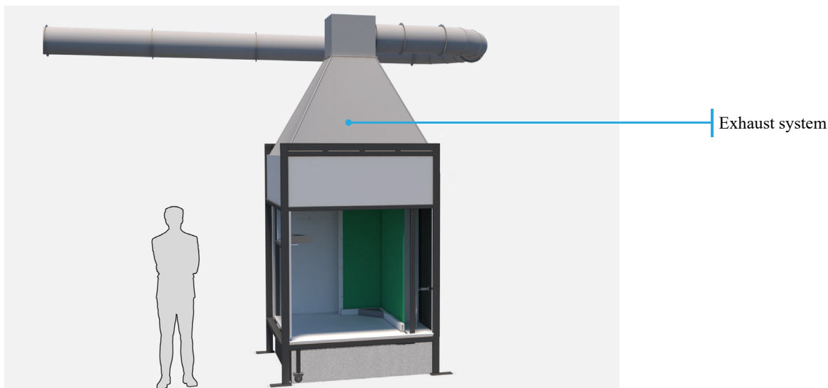
Figure 5.4: Depiction of test apparatus for BS EN 13823
