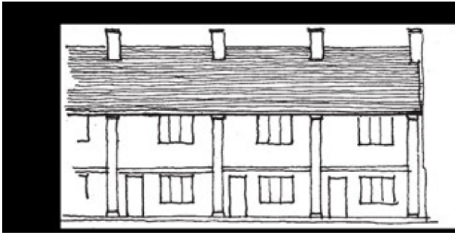
Front elevation with larger openings and facade subdivided to emphasise individual houses
