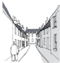
Limiting visual length by taller terminal building
