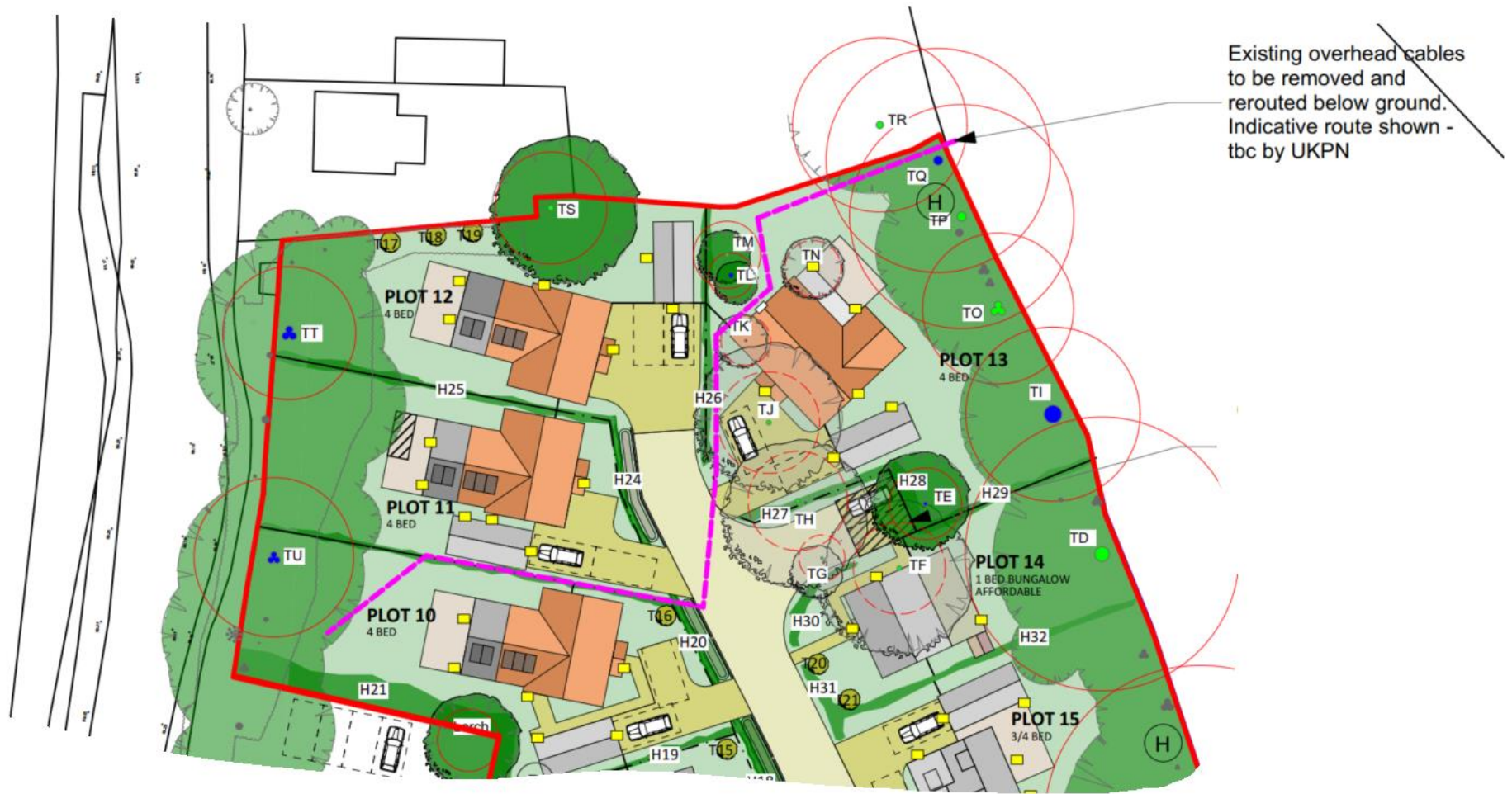
Fig. 2 Extract from the site layout plan showing the proposed diversion of existing overhead power lines.
