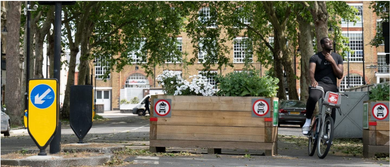
Figure 8: A modal filter in an earlier emergency LTN in Lambeth (London Borough of Lambeth)
