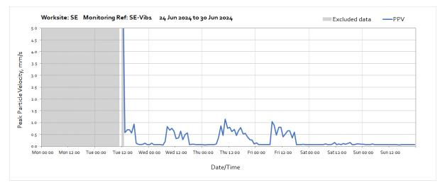
Note: Data excluded throughout the week due to spurious data. Missing data between 11:00 and 12:00 on Tuesday 25<sup>th</sup> June was due to monitor retrieval for repair. A new vibration monitor was installed at 12:00 on Tuesday 25<sup>th</sup> June.
