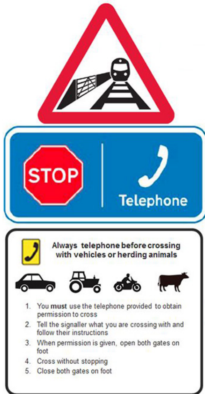
Figure 17: New UWC-T sign being trialled by Network Rail
