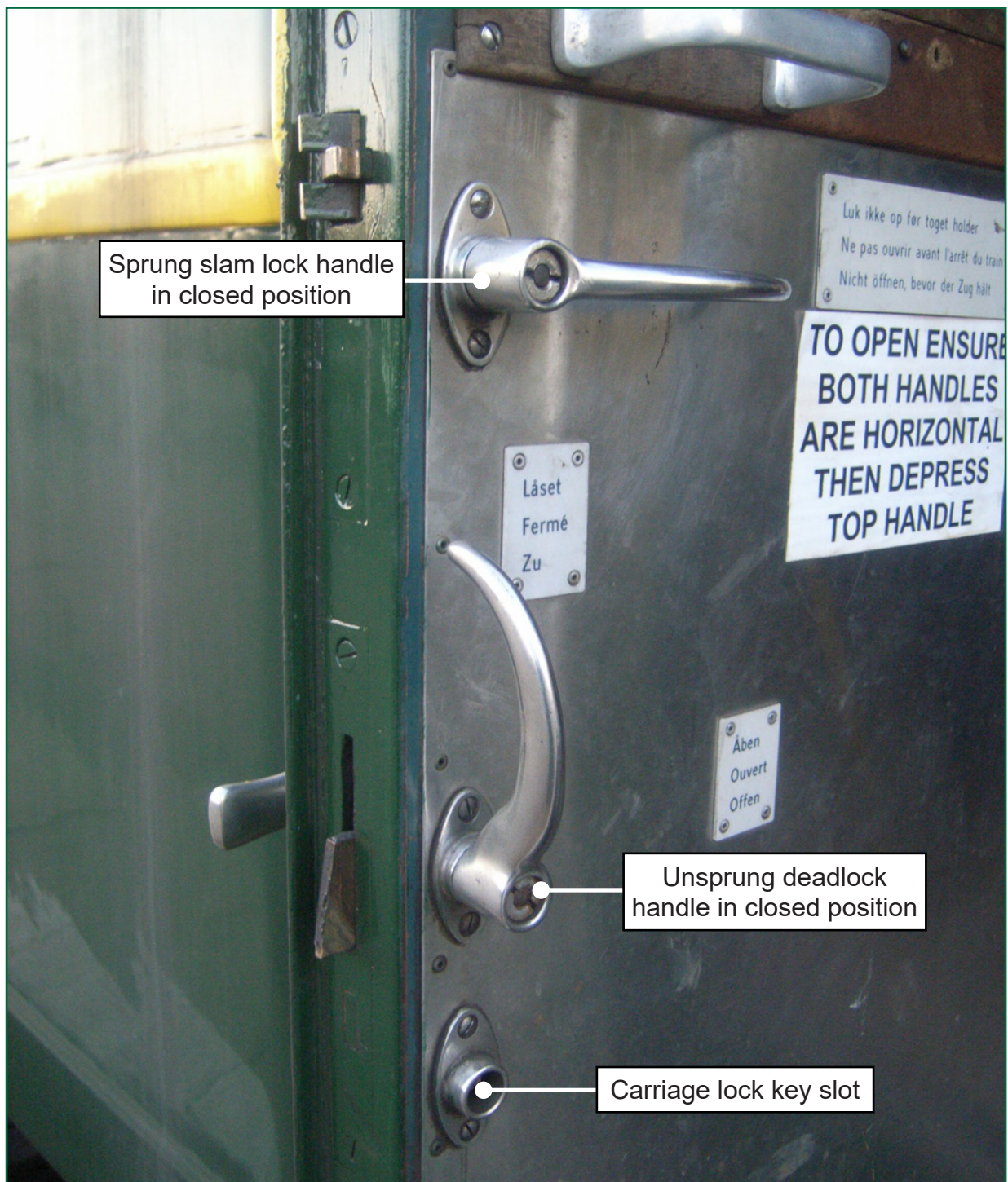
Figure 3: Incident door showing slam door and deadlock handles
