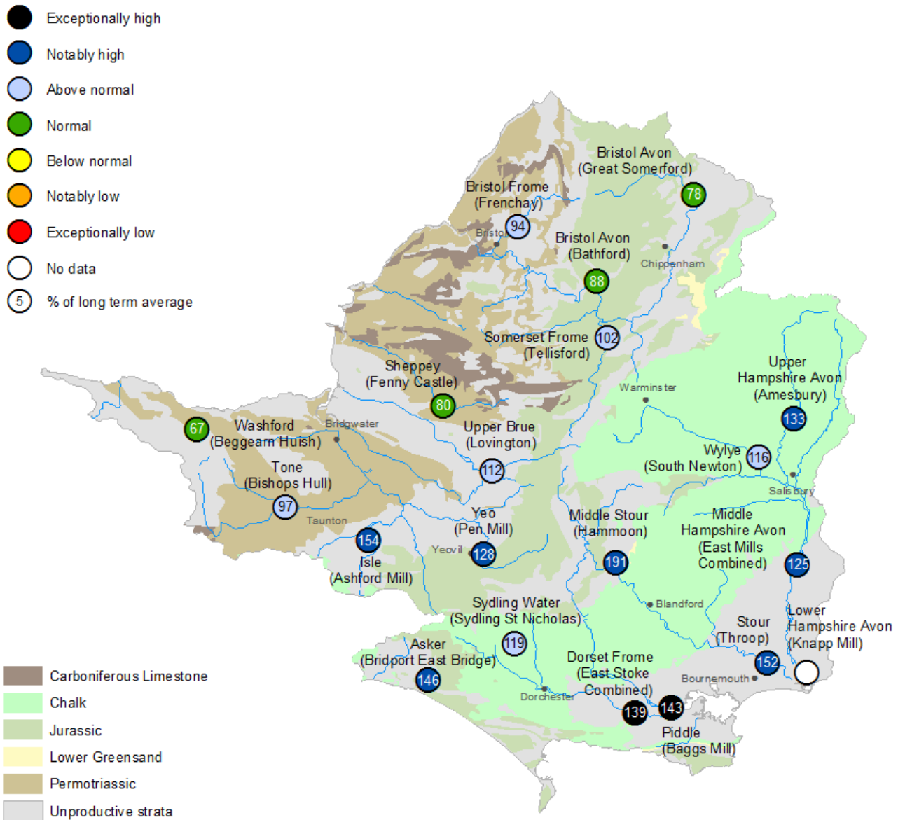
Figure 4.1: Monthly mean river flow for indicator sites for July 2024, expressed as a percentage of the respective long term average and classed relative to an analysis of historic July monthly means Table available in the appendices with detailed information.
