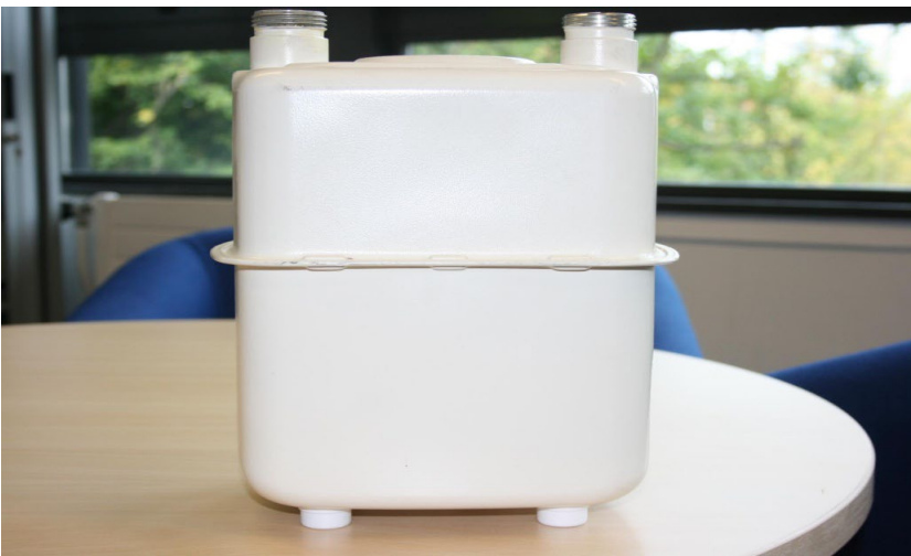
Gas meter – No rust over meter band
