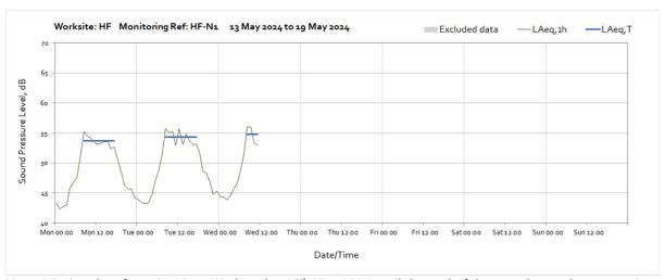
Note: Missing data from 12:00 on Wednesday 15<sup>th</sup> May 2024 until the end of the month was due to monitor retrieval after failed field calibration.
