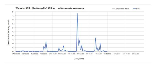
Note: High vibration levels at 08:00 on the  $30^{th}$  of May were due to topsoil stripping works taking place close to the monitoring station.
