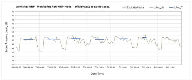
Note: Missing data between 12:00 and 13:00 on Sunday 7<sup>th</sup> May was due to monitor configuration error.
