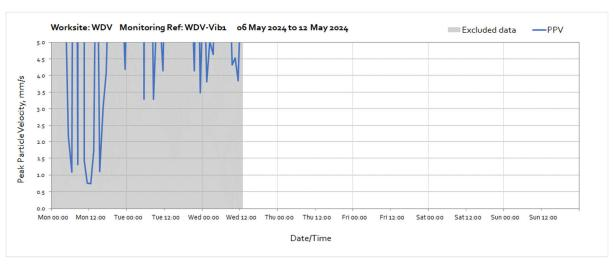
Note: Monitor data excluded due to erratic readings. Monitor retrieved for investigation at 13:00 on Wednesday  $8^{th}$  May due to erratic readings.
