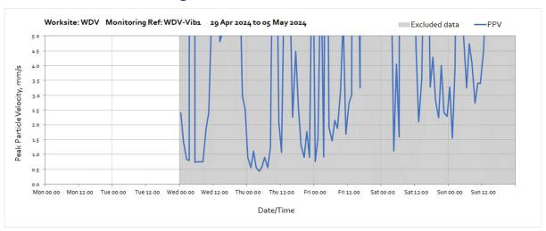
Note: Monitor data excluded due to erratic readings.
