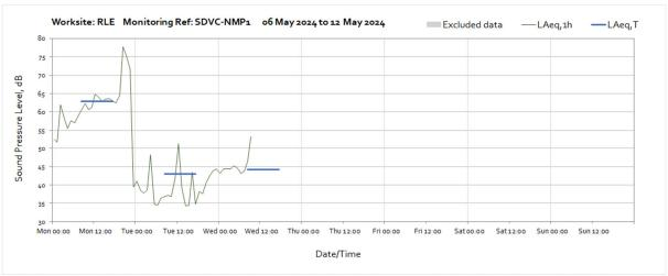
Note: Missing data from 10:00 on Wednesday 8<sup>th</sup> May until 12:00 on Friday 17<sup>th</sup> May was due to monitor retrieval for repair after a microphone fault during field calibration on Wednesday 8<sup>th</sup> May.
