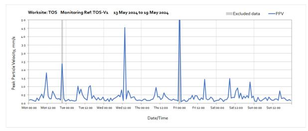
Note: High vibration levels between 13:00 and 14:00 on Wednesday 15<sup>th</sup> of May was due to cage fabrication, shuttering and plant movement undertaken close to the monitor.
