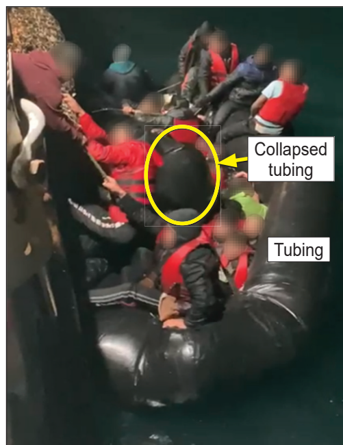
Figure 2: Inflatable migrant boat Charlie alongside Arcturus , with its flooring missing and tubing collapsed together
