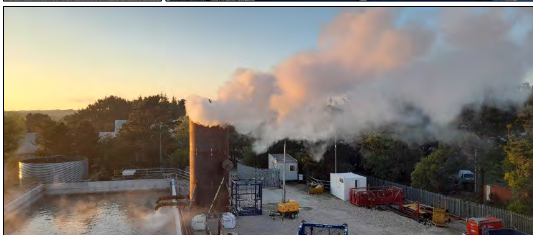
During testing, steam was visible from both the steam separator and outflow into the lagoon
