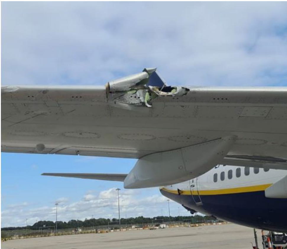
Figure 2 Damage to the aircraft
