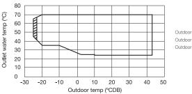
Outdoor temp. -25°CDB/Outlet water temp. 45~65°C Outdoor temp. -20°CDB/Outlet water temp. 35~70°C Outdoor temp. 43°CDB/Outlet water temp. 24~70°C
