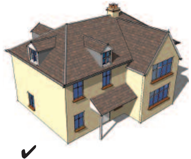
Examples of subservient dormer windows in a detached house
