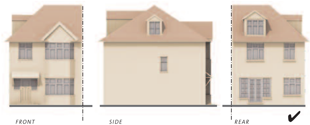
An example of subservient dormer windows in a semi-detached house
