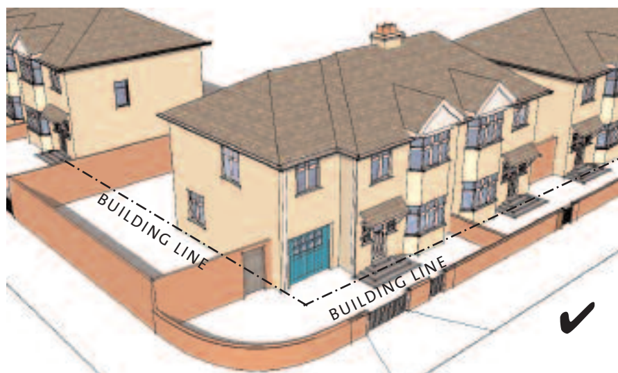
Side extensions at corner locations should respect the established building lines and not encroach beyond them
