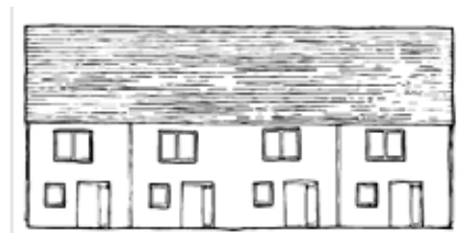
Front elevation with minimum openings. Illusion created of larger houses: door opening could control windows to either side
