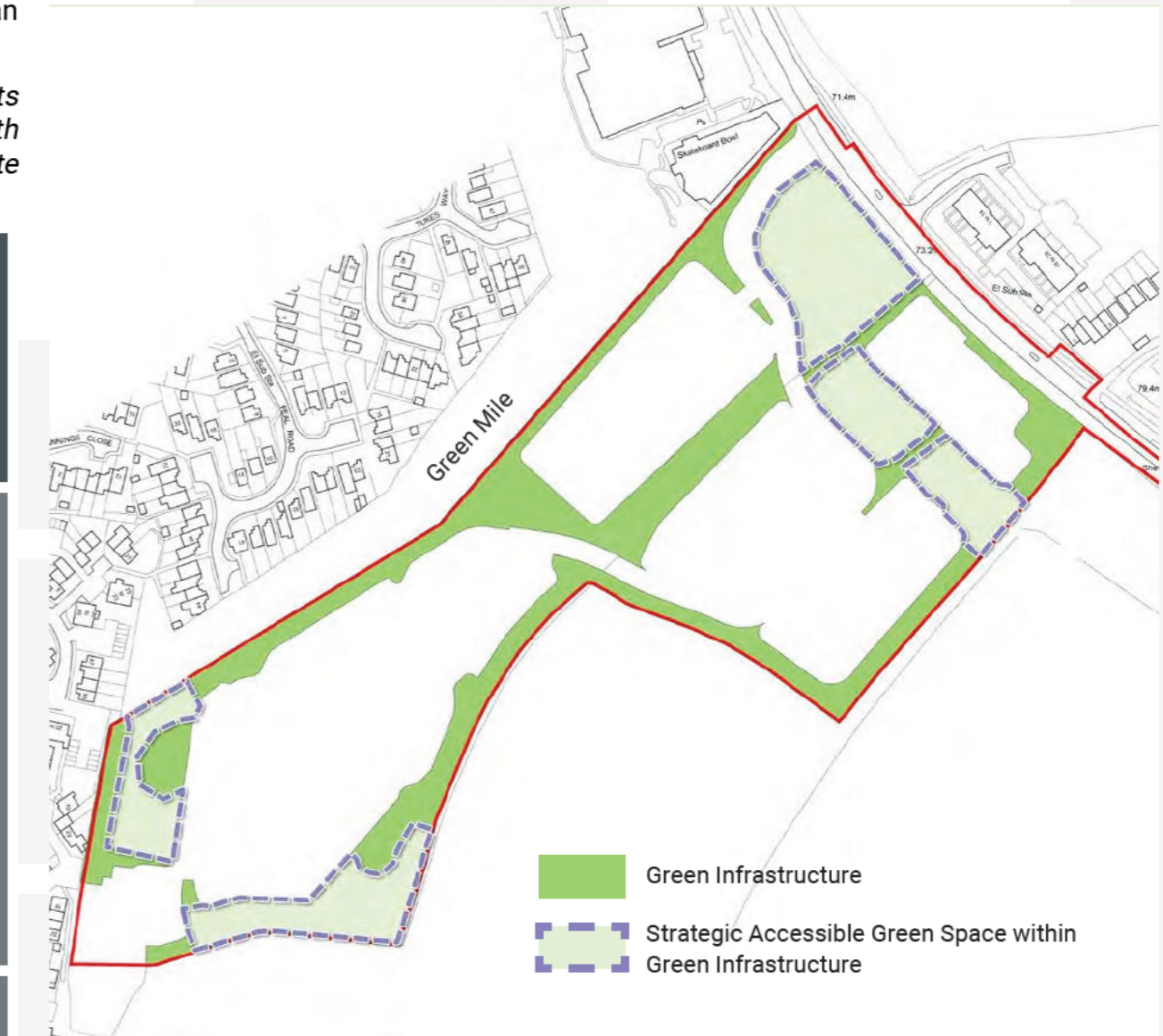
Indication of 1.3Ha minimum required provision of Parks, Gardens, Amenity plus Natural and Semi-Natural Accessible Green Space overlaid upon Green Infrastructure Plan
