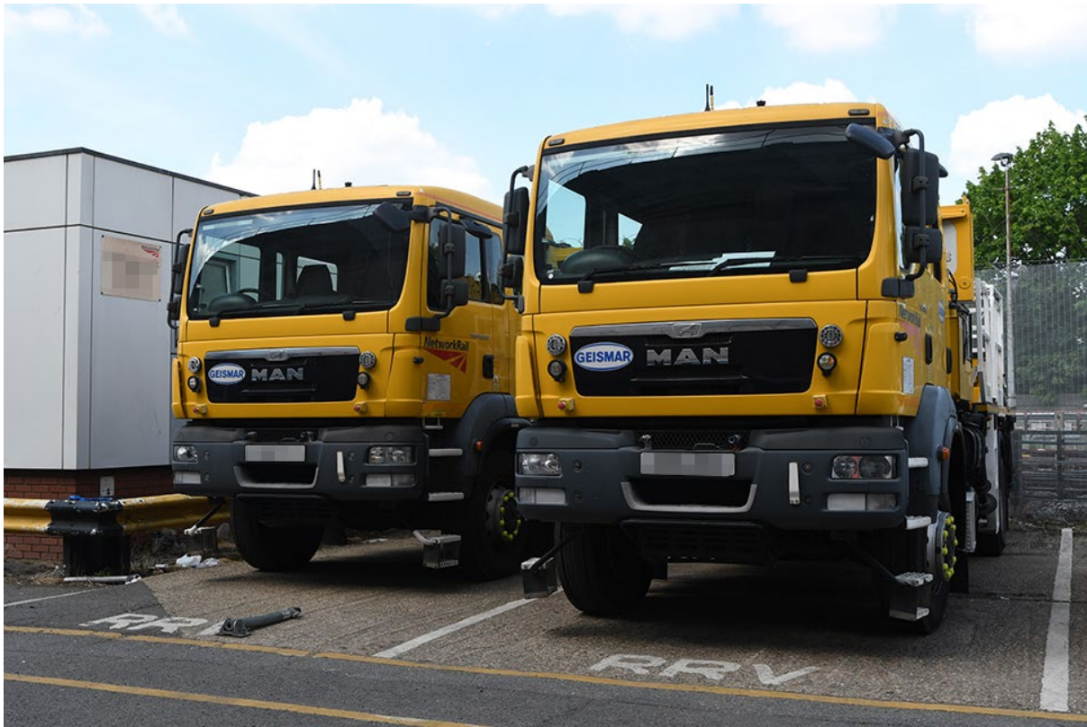
A pair of road-rail vehicles with mobile elevated work platforms as used on the WCML for OHLE equipment work.
