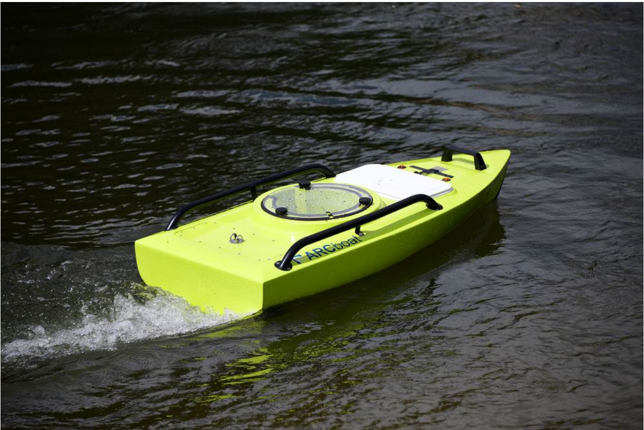
Photograph 3: Remote controlled boat used for bathymetric surveys (source: HR Wallingford, 2022)
