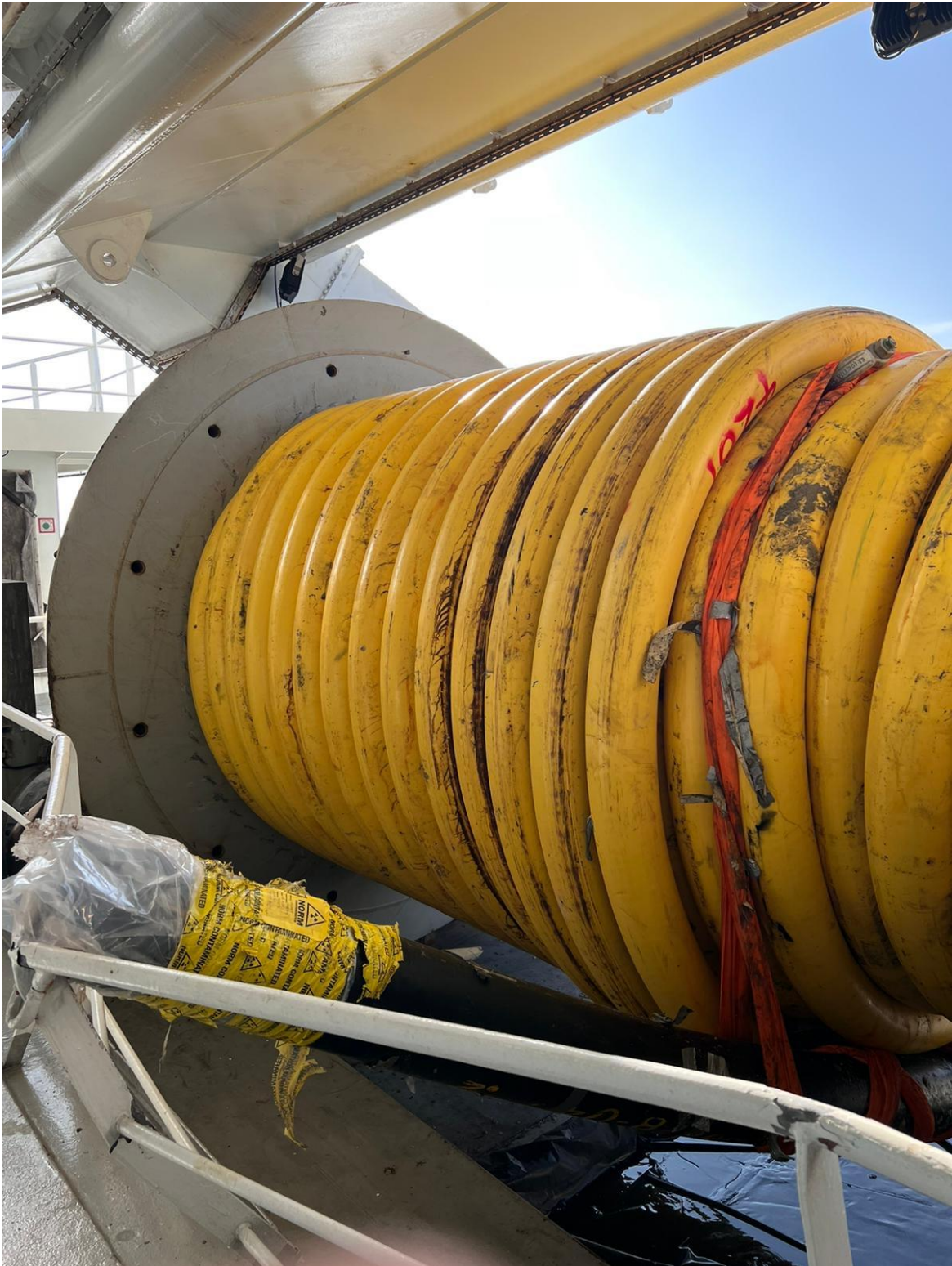
Figure 9.4.1: Umbilical riser on AHV drum
