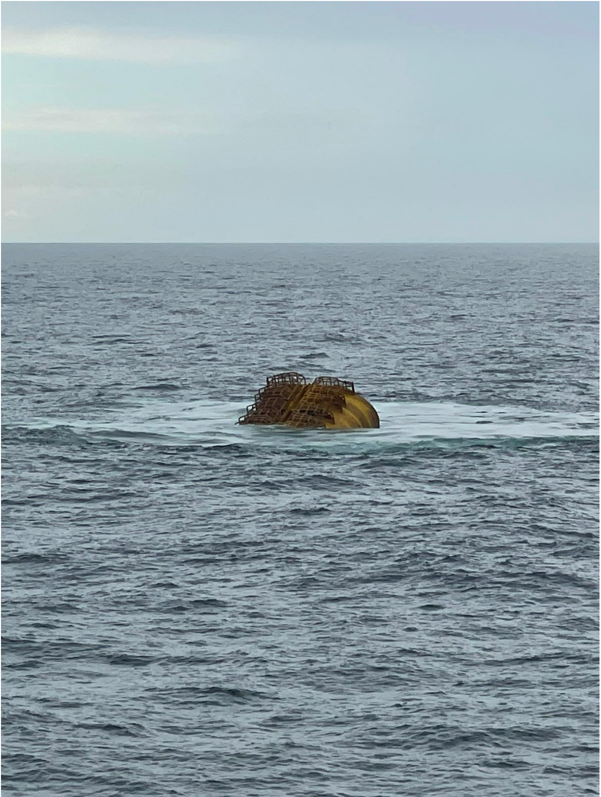
Figure 9.5.2: Mid-Water Arch stabilising from having been released
