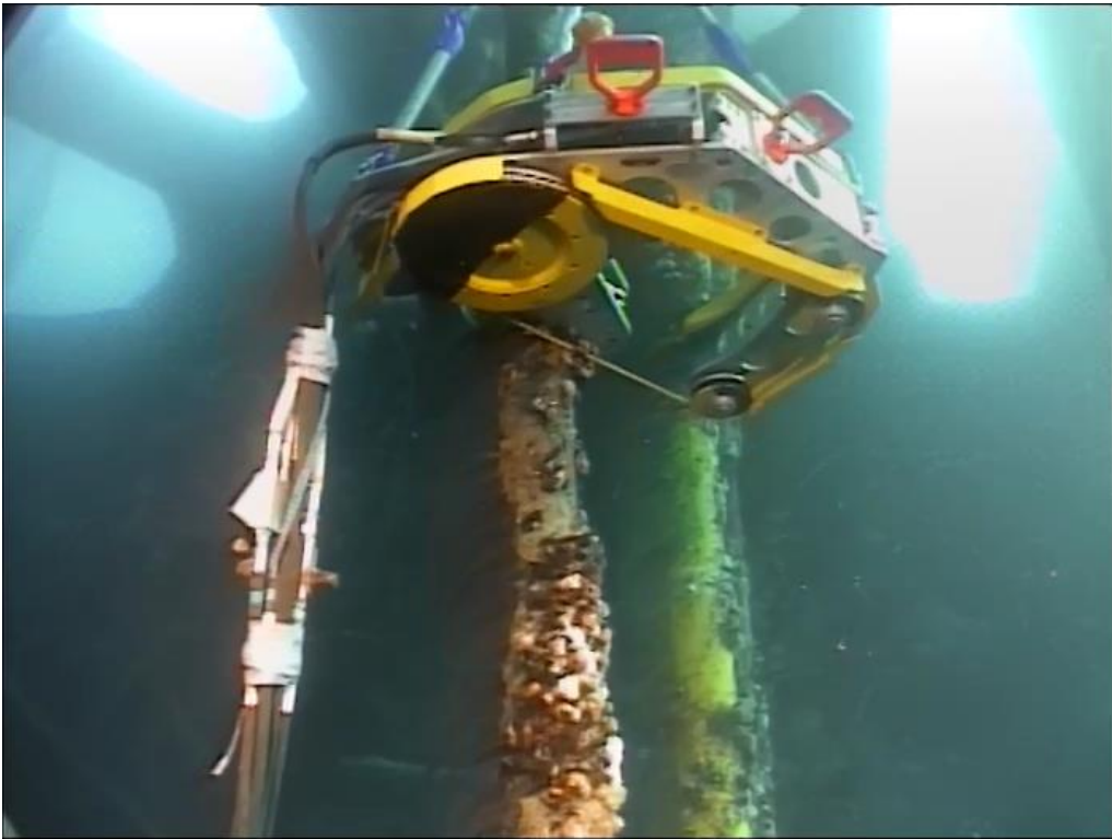
Figure 9.3.1: DWCM in position on riser PL2574
