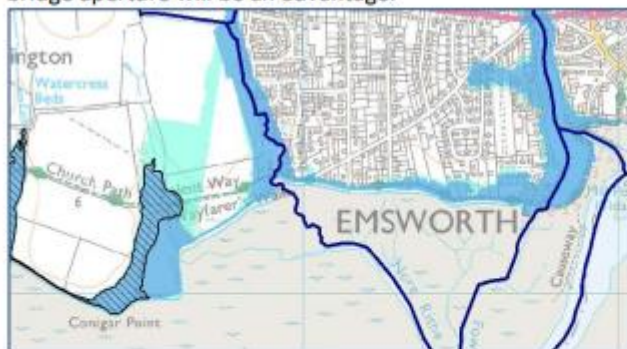
Environment Agency Flood map excerpt. Dark blue line = main river (Includes Nore Farm stream). Blue shading = Flood zone 3
