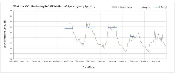
Note: Missing data from the start of the month until 13:00 on Wednesday 10<sup>th</sup> April was due to a loss of power to the monitoring station caused by poor weather conditions preventing sufficient light to reach the solar panel.
