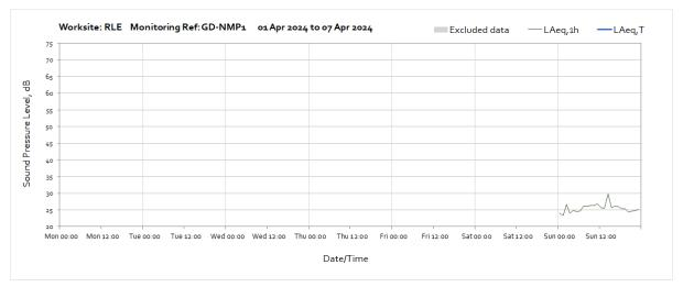
Note: Missing data from the start of the month until 00:00 on Sunday 7<sup>th</sup> April was due to a monitor fault, monitor was sent to supplier for investigation and replaced.
