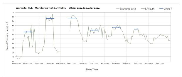
Note: Missing data between 01:00 and 10:00 on Wednesday 10<sup>th</sup>April was due to a loss of power to the monitoring station caused by poor weather conditions preventing sufficient light to reach the solar panel.
