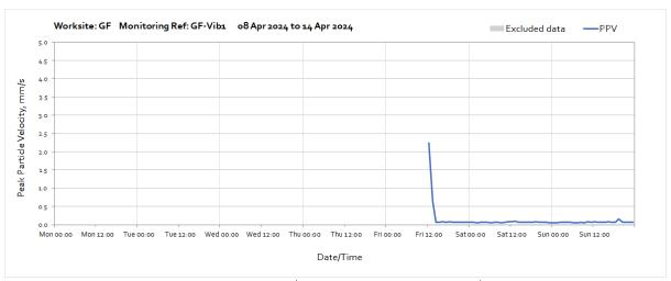
Note: Missing data between 02:00 on Sunday 7<sup>th</sup> April and 12:00 on Friday 12<sup>th</sup> April was due to a loss of power to the monitoring station caused by poor weather conditions preventing sufficient light to reach the solar panel.
