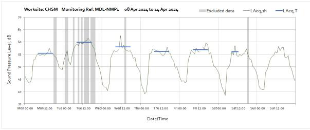
Note: Missing data between 13:00 and 14:00 on Friday  $12^{th}$  April was due to a communication error between the monitoring station and server.
