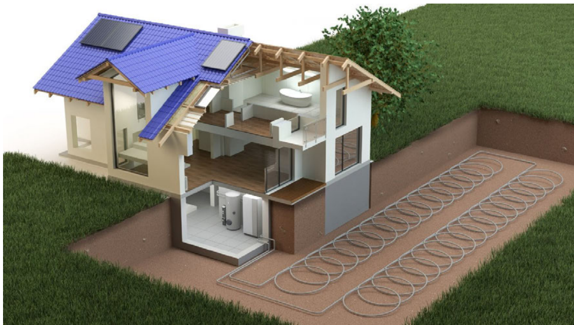
Horizontally sunk ground source heat pump
