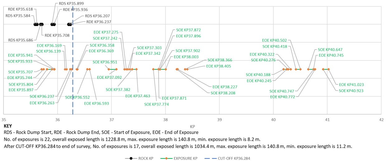
Figure 3.4.5: PL1965 & PL1966 rock vs. exposure detail (2017) 7
