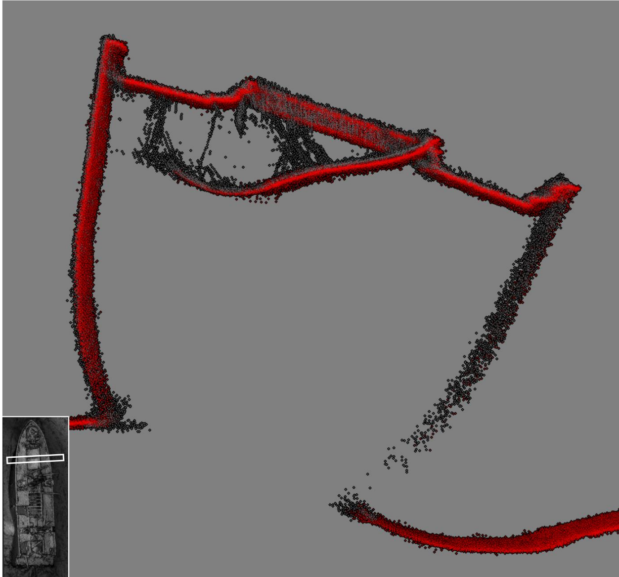
Figure 27. Cross section through the hull at the forward end of no. 1 hatch. Red full survey 2023, grey full survey 2022.
