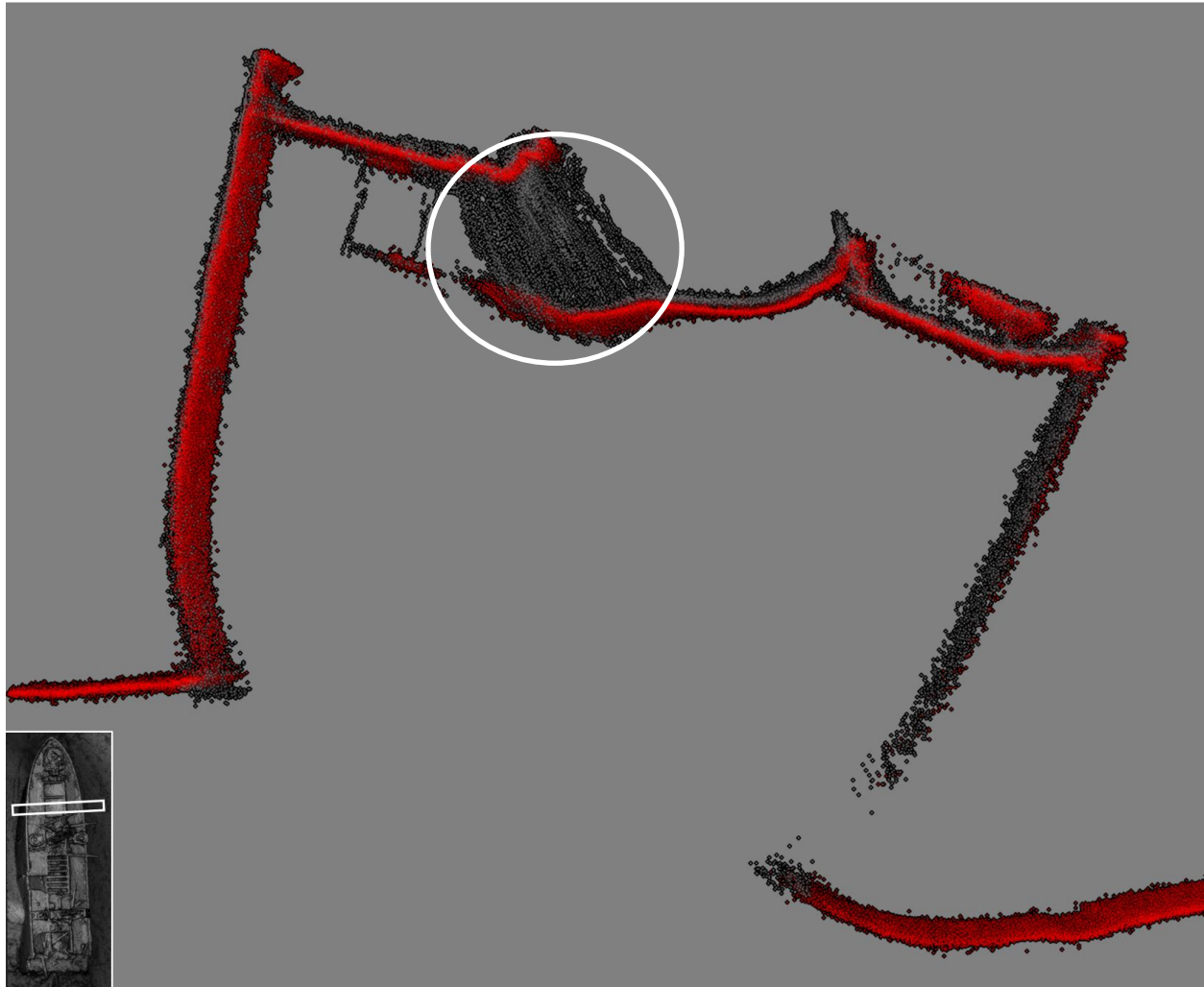
Figure 28. Cross section through the hull at the aft end of no. 1 hatch. Red full survey 2023, grey full survey 2022. Circled is an area where there is a large difference between the surveys, most likely noise in the 2022 survey.
