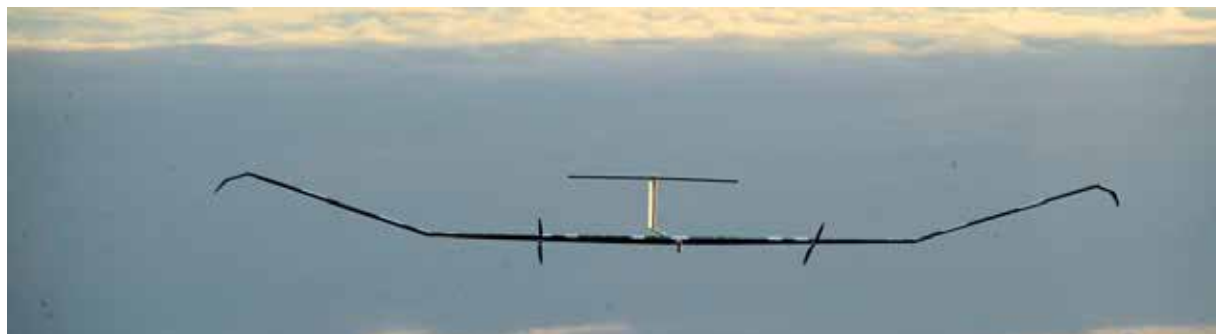
The Zephyr high altitude pseudo satellite has the ability to remain airborne for 14 days
