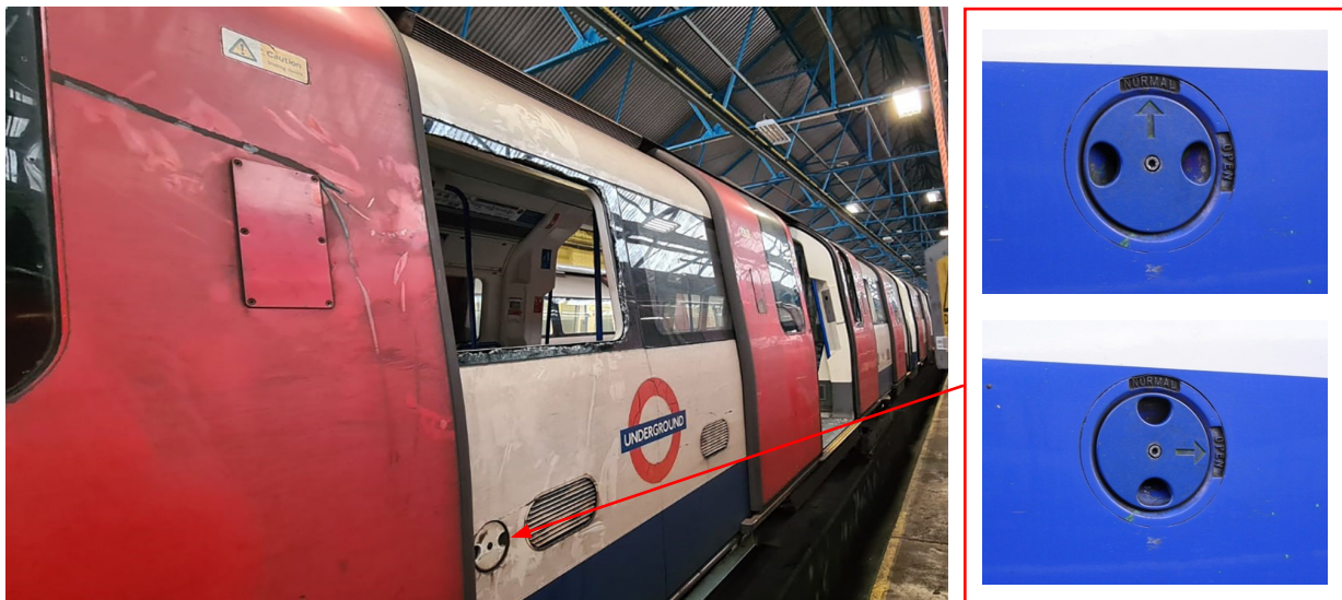
Figure 7: Train 065 at Golders Green depot after the incident. Inset images show ODOD in normal / doors closed (top inset) and open / doors open (bottom inset) positions. Images courtesy of LUL.
