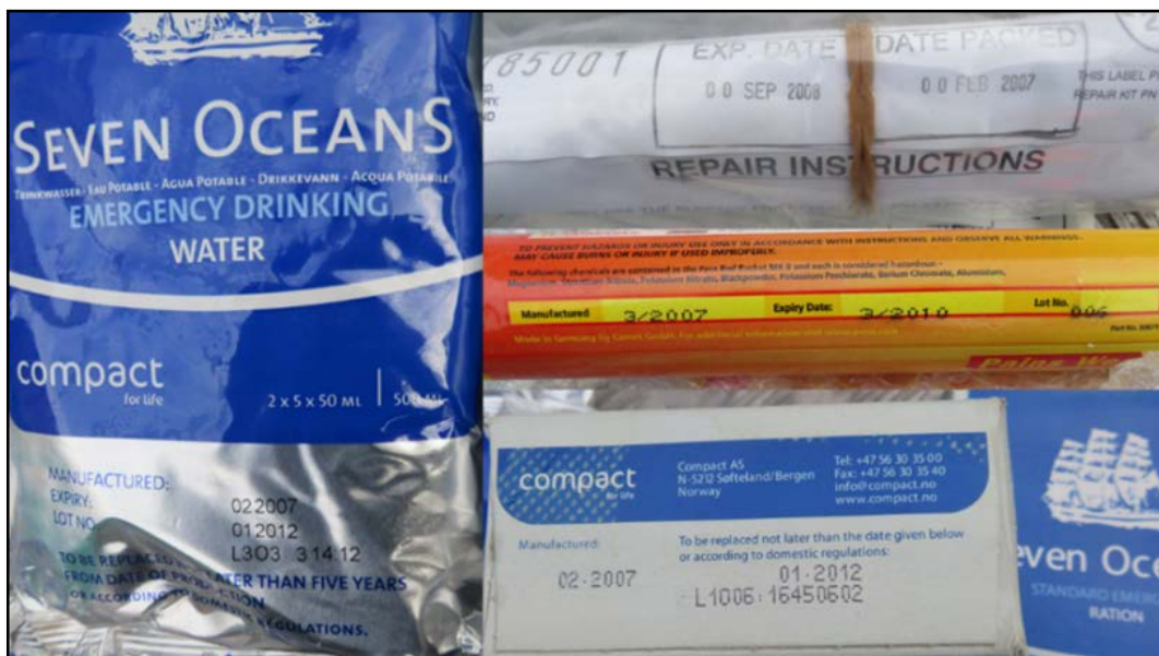
Figure 2: Examples of the expired consumable items in Piedras's starboard liferaft
