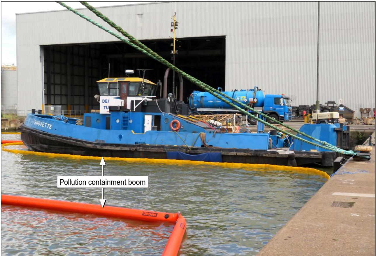
Figure 7: Pollution booms deployed
