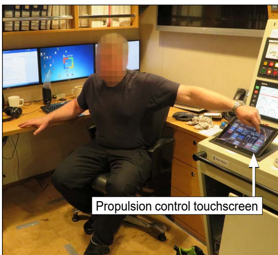
Figure 4: Engineer reaching across to the propulsion control touchscreen
