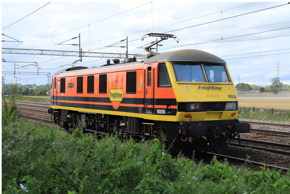
Figure 5: Class 90 locomotive during the test run (courtesy of John Neave).
