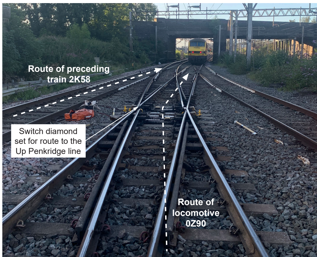
Figure 8: The final stopping position of the locomotive (courtesy of Network Rail with RAIB annotations).
