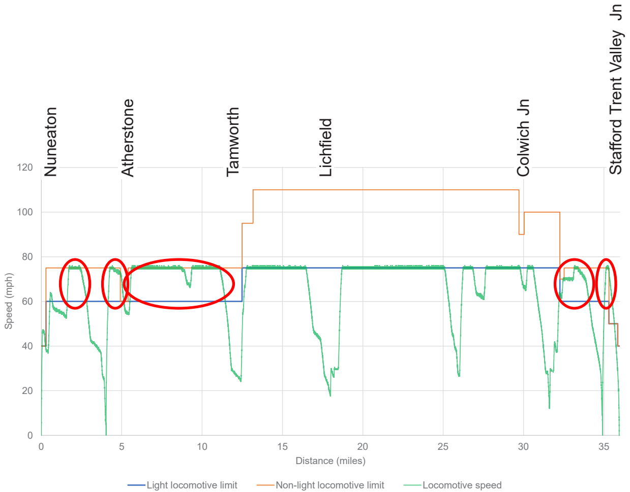
Figure 13: Locomotive speeds on the northbound journey from Nuneaton to Stafford Trent Valley Junction No. 1.
