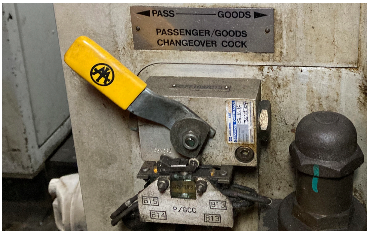
Figure 16: Passenger/Goods changeover switch on the class 90 immediately after the incident (courtesy of Freightliner).
