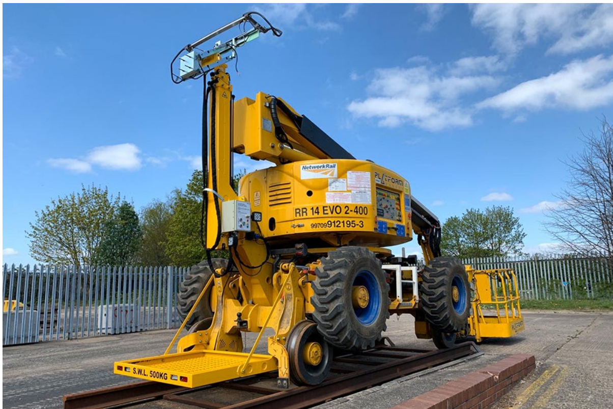
An RRV of the same type as the machine involved in the accident, with deployed carry deck nearest the photographer and operator's basket at the opposite ('trailing') end. (Courtesy of SPL Powerlines UK Ltd.)
