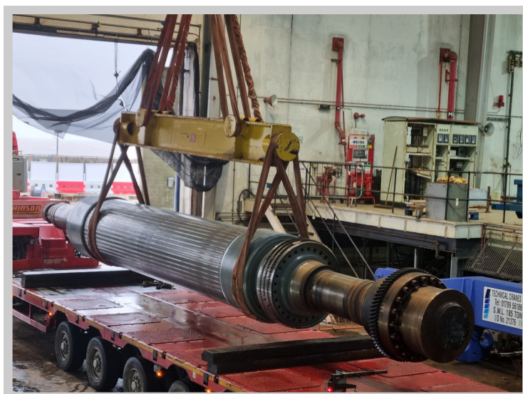
Figure 12: Despatch of Turbine Rotor
